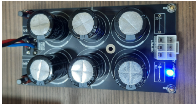
Extra capacitance PCB, accepts capacitors from 25mm up to 35mm
